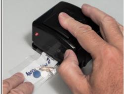
Place the open end of the pouch into the sealer and press down. The light will come on for 3 seconds, when the light goes out the pouch will be sealed.
