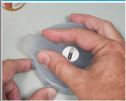
Snap on the filling tray lid, the lid chute should be over the first slot of medications.
